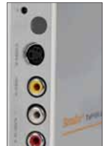
Ports include inputs for S-Video, composite and stereo audio.
